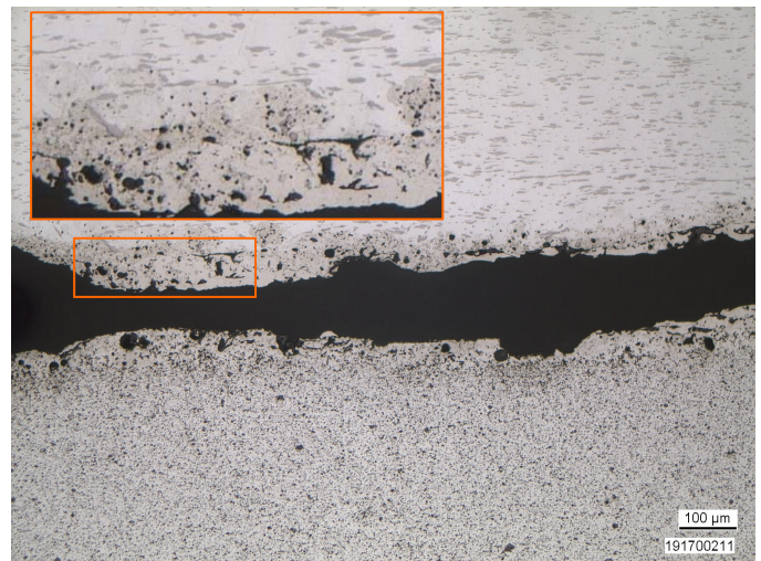
Figure 10. Cross section of AgNi10 (upper) and Ag-SnO 2 88/12 SPW7 (lower) after test
